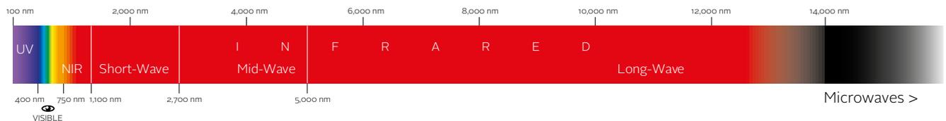
It covers a spectrum from 0.75  $\mu\text{m}$  - 14  $\mu\text{m}$  wavelength and is separated into near-infrared (NIR), short-wave infrared (SWIR), mid-wave infrared (MWIR), and long-wave infrared (LWIR). To detect light in these different spectral ranges specific detector materials are used. For example, silicon-based standard CCD/CMOS sensor can detect light only up to 1,100 nm, because silicon gets transparent beyond this wavelength.
