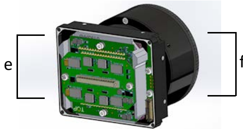
Figure 15: Front assembly overview: sensor unit and lens mount
