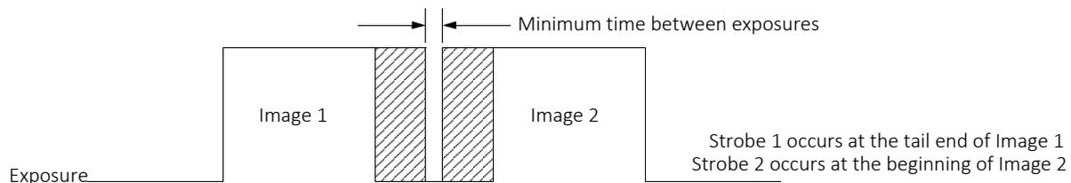
To set strobe(s), there are two possible options, as determined by the camera type. Both options use the camera `SyncOut1/2/3` signal to trigger a strobe.
